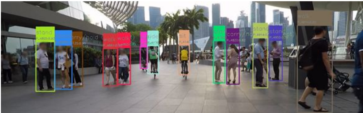
Figure 7. The actions detected for a typical scene. The tally of the above scene is “stand”=5, “walk”=3, “ride”=2, “sit”=1, “run/jog”=0. Any other actions that are not part of the 5 categories are not recorded. Source: authors.
